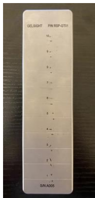
(a) Groove depth reference specimen RSP-GT01
